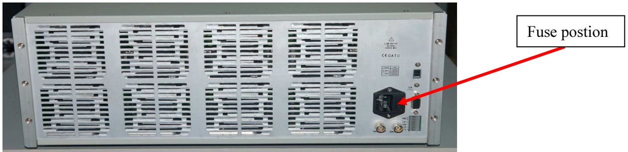
Picture 3.1 Fuse Location
